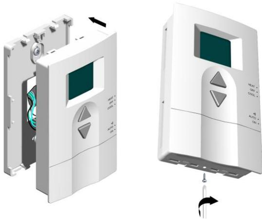
Fig. 5. Installing and securing the thermostat
